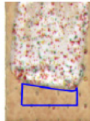
Poor Deposit (within central region, large surface area of a reduced height - blob analysis)
